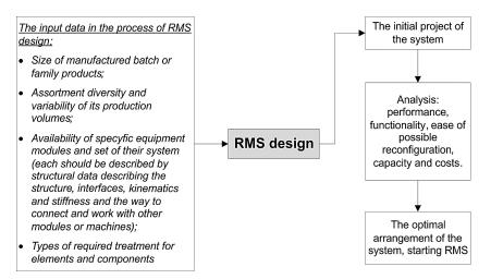
Fig. 3. RMS design stages (own study based on [9])
